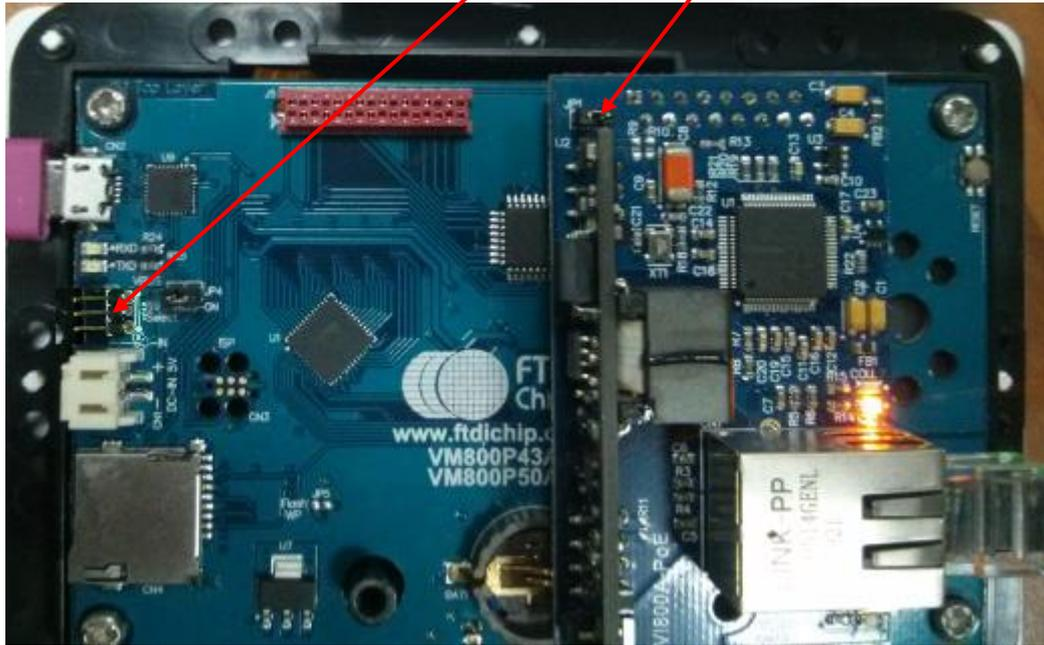
**Figure 2-11 Complete Hardware setup for PoE**
