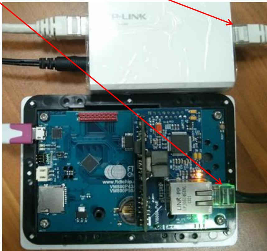
**Figure 2-8 POWER+DATA OUT connection**
