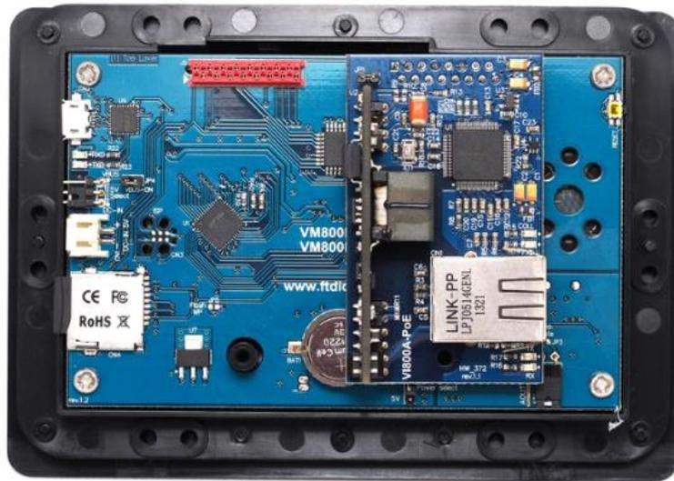
**Figure 2-3 POE connected to VM800P**
