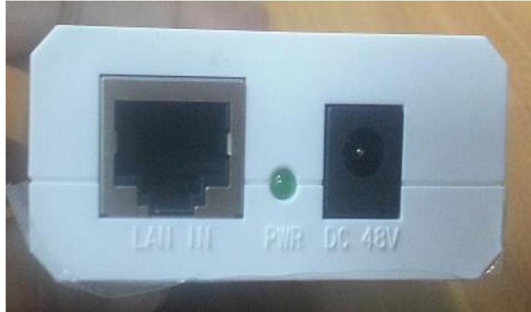
**Figure 2-5 LAN IN port and PWR connector**
