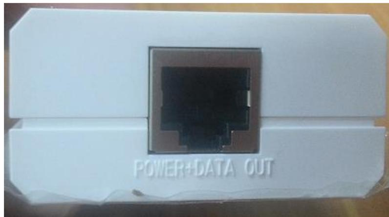
**Figure 2-6 POWER+DATA OUT socket**
