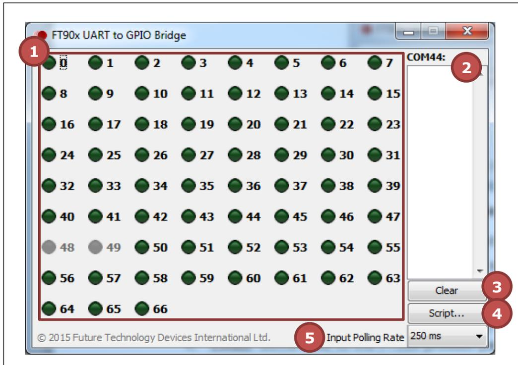
**Figure 2: GPIO Control Window Example**
