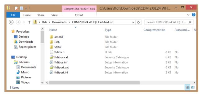
The ftdibus.inf and ftdiport.inf files can be edited to change driver settings such as Vendor ID (VID), Product ID (PID), and Latency etc.
